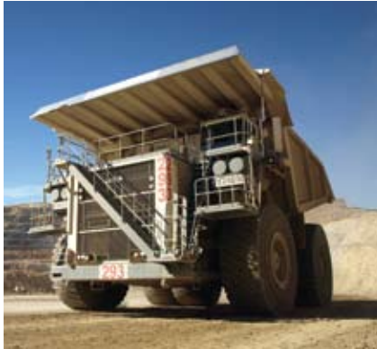
Mining Haul Truck outfitted with two Donaldson SSG Air Cleaners
